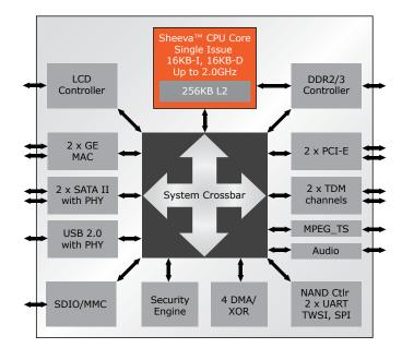
Fig 1. 88F6282 SoC Block Diagram
