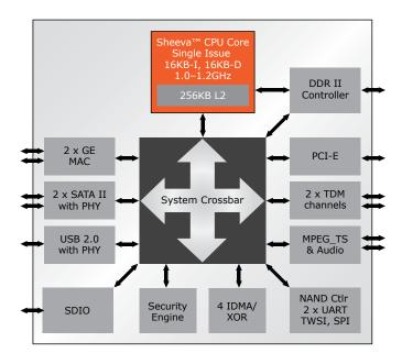
Fig 1. 88F6281 SoC Block Diagram
